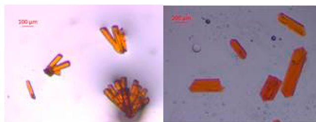
Figure 1. Microscopic images of RWLC-1 (left) and RWLC-2 (right). Images were obtained from a Zeiss SteREO Discovery V8 Microscope with an Achromat S 1.0× FWD 63 mm objective and 2× or 1.25× zoom. Microscope is equipped with a Digital Microscopy CMOS Camera AxioCam ERc 5s, 1×.
